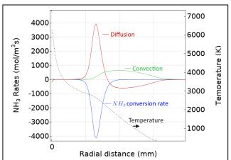
**Figure 1**. Contributions to the local balance of  $NH_3$  production and loss. Chemical reactions in blue, radial diffusion in red, convection in green. The local temperature as well as the sum is also indicated. Values plotted at a cutline halfway between the electrodes for a flowrate of 15 NLM and an SEI of 35 kJ/mol.
